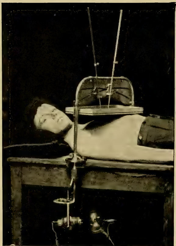
PLATE 79.—Remy Localizer. Second position. Move the tube horizontally to the focus for the second shadow on the screen and push down the second rod to meet the centre of this shadow. The two rods then are the equivalent of the axis of the rays from the two foci.
